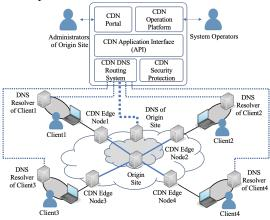
Fig. 1. Architecture of the Content Delivery Network
